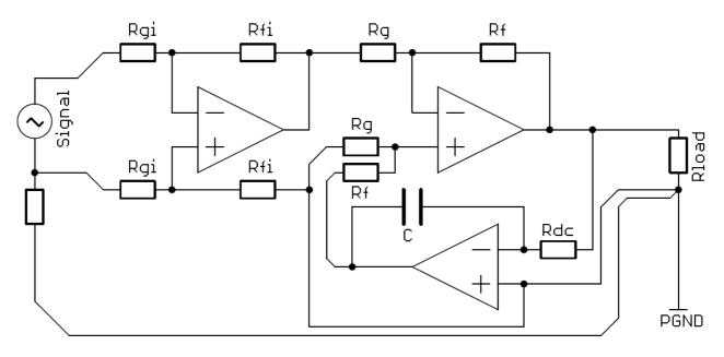
fig.7 simplified grounding sheme with DC-Servo
