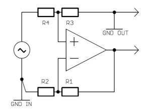
fig.5b pseudo differential GND converter
