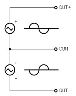
fig. 1: differential signal
