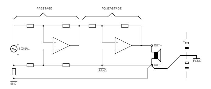
fig. 6: simplified amplifier using pseudo differential connections
