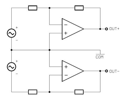
fig. 4: differential signal stage
