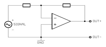
fig. 3: single ended signal stage
